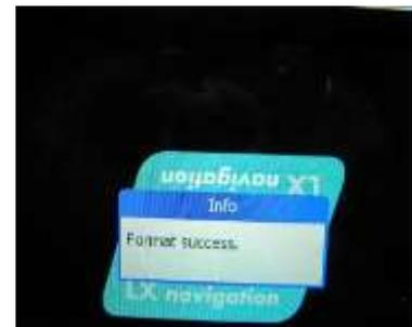
System reset will be executed automatically without any further assistance. The process termination is visualized with **Format success** message.
